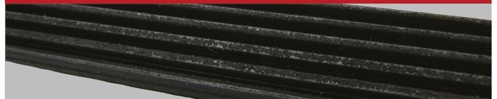
**(C1) Bubbling of elastomer compound and decomposition of vulcanization**
