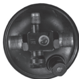
RD12072 Diameter: 3" Legth: 8-1/4" In/Out: 3/8" x 3/8" Male O-Ring Schrader Valve Fuse Plug Moisture Indicator OE# 61506-3402
