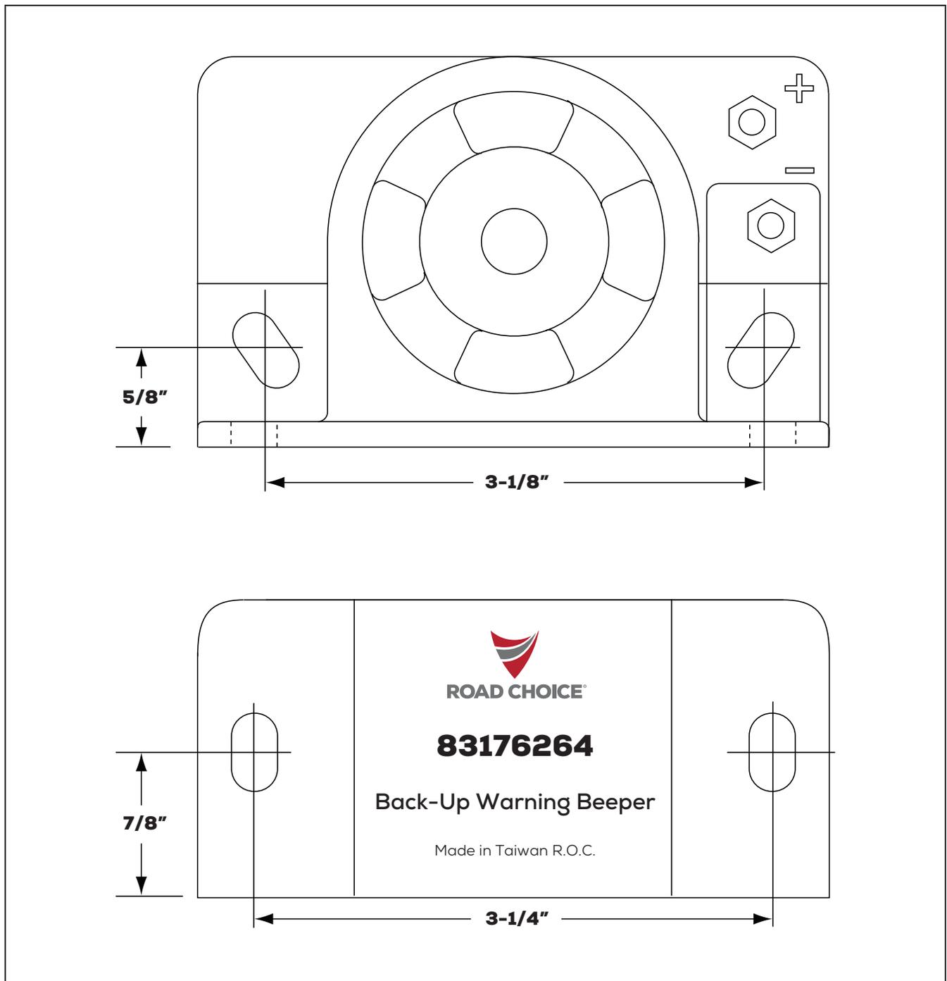
Select a mounting location near the rear of the vehicle that will provide protection from flying objects while allowing an unobstructed sound from the vehicle.
